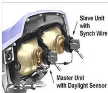
On most models, access to the 3-pin connectors of the headlamp bulbs is possible simply by reaching it from underneath the front fairing or from behind the dash. There is usually a rubber splash cover over the pins of the bulb, which has to be peeled back.
