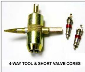
If you felt that it was hard to thread it for the last couple of turns, or you need at least a ½ more turn to seal it up; remove the sensor and use the 4-Way tool to chase and clean the threads of the valve-stem.
