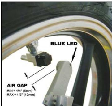
As shown here the antennae of the Transceiver should line-up with the face of the Sensor on the wheel – with about a 1/4" (6mm) of air gap.
