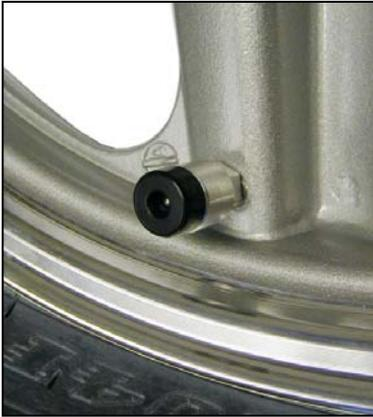
Installing TPM-40 sensors requires them to be fully threaded-in on the tire valve to provide secure sealing.
